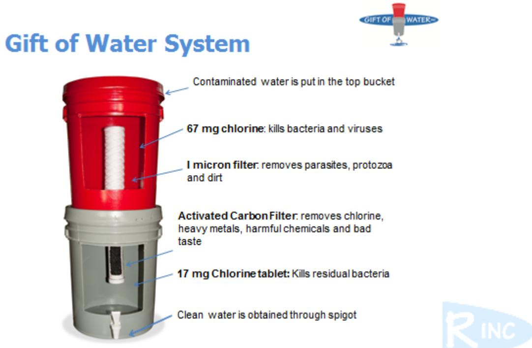
The Gift of Water filtration system incorporates a multi-barrier approach that leads to high quality treated water.
